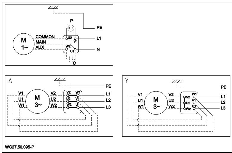
230/400 V three phase motors are connected in delta for 230 V and in star for 400 V.
